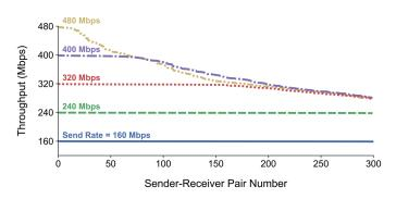
**Figure 4:** The distribution of achieved network throughputs between pairs of workers at five different send rates on AWS Lambda. Each point corresponds to a sender-receiver pair, and the lines are labeled with their corresponding send rates.
