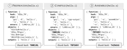
**Figure 3:** An example of gg IR consisting of three thunks for building a "Hello, World!" program that represents the expression Assemble(Compile(Preprocess(hello.c)))  $\rightarrow$  hello.o. To produce the final output hello.o, thunks must be forced in order from left to right. Other thunks, such as the link operation, can reference the last thunk's output using its hash, T42hGtG. Hashes have been shortened for display.
