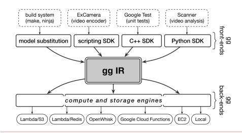
**Figure 1:** gg helps applications express their jobs in an intermediate representation that abstract the application logic from its placement, schedule, and execution, and provides back-end engines to execute the job on different cloud-computing platforms.
